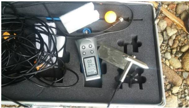
Gambar 3. Alat pengukuran Debit Air (Current meter).
